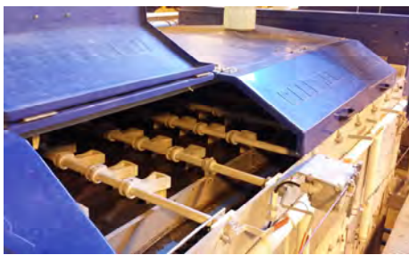
View of upper portion of a belt filter press during gravity separation.
