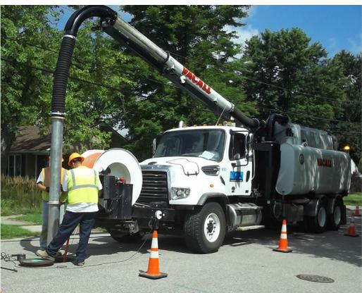
YCUA crews perform periodic sewer main inspections using remotely-controlled video cameras. If there are obstructions such as roots or grease, the sewer main is cleaned using a sewer
